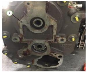
2. Install the HST unit on the gearbox using Suitable lifting device.
